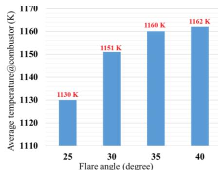
Fig. 11 – Average temperature distribution in the whole combustor
