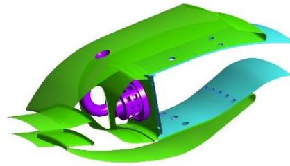
Fig. 1 – 3D CAD model of combustor
