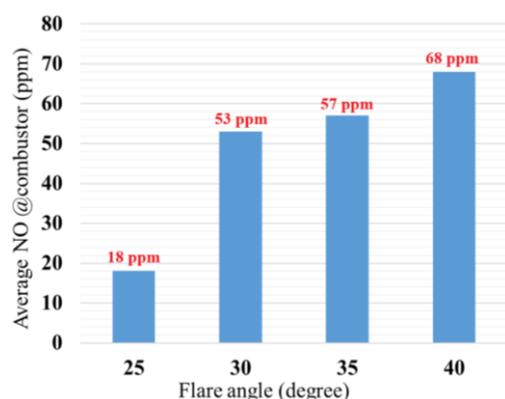
Fig. 12 – Average NO distribution in the whole combustor
