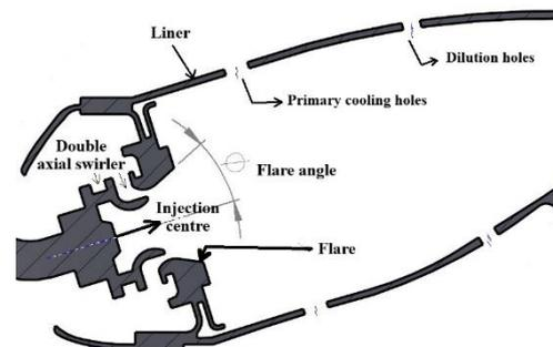
Fig. 3 – Cross section of structure of the double axial swirler including the liner schematic
