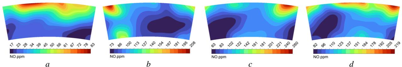
Fig. 9 – Contour of NO distribution at the outlet of combustor in various flare angle:
