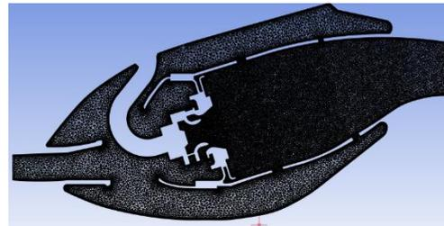
Fig. 2 – 2D view of the cross-section meshes
