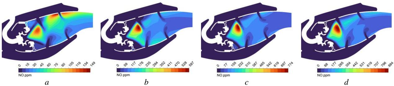
Fig. 8 – Cross section of NO distribution contours along the combustion chamber in various flare angle:
