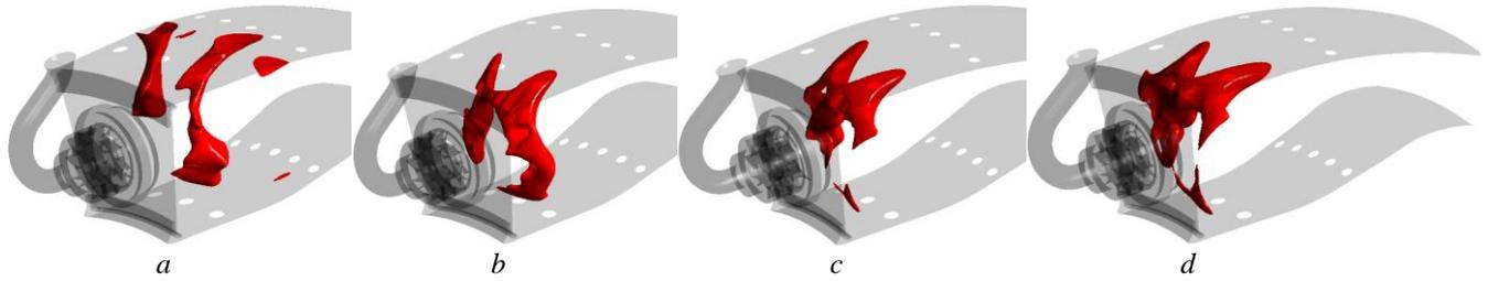
Fig. 6 – Iso surfaces of maximum total temperature in flame tube in various flare angle:
