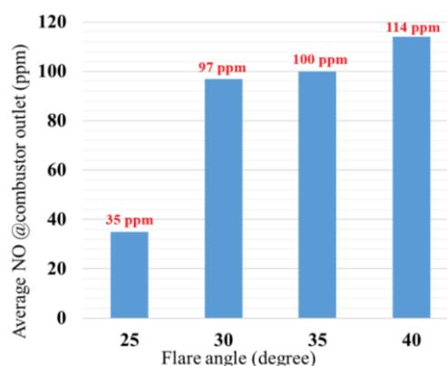
Fig. 13 – Average NO distribution at the outflow combustor
