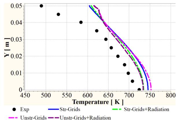
Fig. 4 – Exit gas temperature distribution obtained at the outlet of combustor in real experiment done by Ghose P. et al. [8] and numerical experiments done by Masoud Hajivand (2021) [9], including structured and unstructured grids, with and without radiation effect
