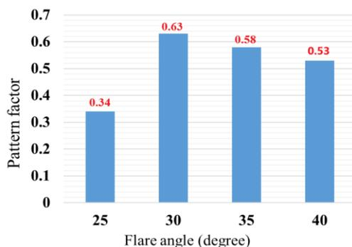
Fig. 10 – Pattern factor for the various flare angle
